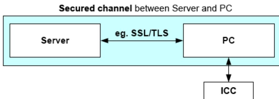
In the above example (taken from EN 14890-2), client/server authentication establishes a secured channel between a remote server and a PC. The ICC will be used as a cryptographic toolbox in order to provide the cryptographic functionality to the PC. If a process needs a certificate from the card that is not provided by OpenPGP (e.g. x.509), then it can be stored in the DO 'Cardholder certificate'.
